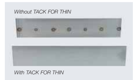
The difference in the tack welds is clearly visible. TACK FOR THIN was used to weld the piece on the bottom, and regular TIG was used on the piece on the top.
